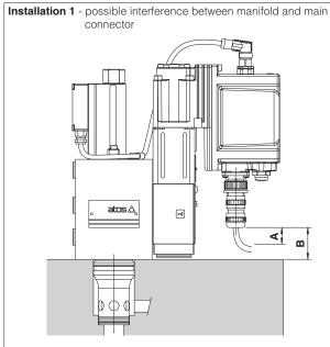
A = 15 mm space to remove the 7 or 12 pin main connectors
