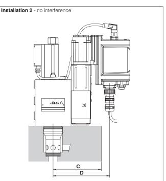
$\ensuremath{\textbf{C}}$  = Max manifold dimension to avoid interference with the main connector, see below table
