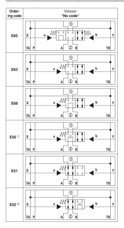
$^{1)}$  Opening cross-section in spool position "a" (A2  $\rightarrow$  B2) = 50  $mm^2$
