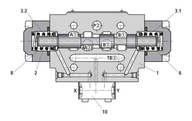
Valves of type Z4WH are directional spool valves with hydraulic actuation. They control the start and stop of a flow.
