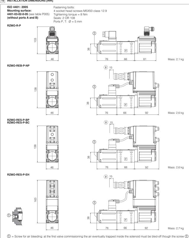
2 = Space to remove the 7 or 12 pin main connector. For main and communication connectors see section [12], [13]
