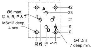
Valve mounting S.H.C Screws M6x70L (4 nos.) Grade 12.9. Tightening torque 16 Nm.
