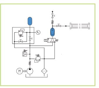
In case of leaking pipe systems, pressure tests (for instance for high-pressure pipes) are mostly used with water which is less contaminating than oil. In order not to have to build stainless-steel pumping units a standard hydraulic unit connected to a transfer accumulator is used (an additional standard accumulator us used to maintain the pressure and prevent the pump from having to run continuously).
