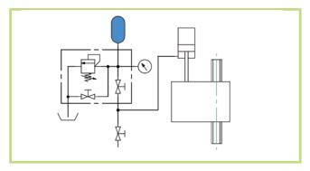
Small dimensions, inertia free accumulators can be used for balancing heads of machine-tools. Compared to a counterweight system with chains, the hydraulic balancing using an accumulator offers the following advantages: weight reduction, lesser vibrations transmitted to the foundations, more compact solution, easier to transport, higher adaptivity thanks to the possibility of varying the gas filling pressure.
