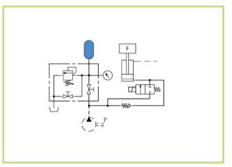
The hydraulic accumulator is used to recover the kinetic energy in a system and return it to the system on demand. This is for instance the case with presses where the press ram pumps the oil back into the accumulator when moving down and reuses the oil when moving back.
