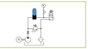
Displacement pumps pulsations generate noise and vibrations and can influence sensitive testing devices. In hydraulic feedback systems servo-valves may start oscillating in an annoying way.
