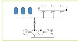
Bearings of big machines such as turbines, compressors and very high capacity water pumps must be constantly lubricated. When mains fail emergency pumps driven for instance by a diesel motor must immediately enter into operation. When starting, the auxiliary pump receives no lubricant during a few seconds. OLAER hydraulic accumulator enter at this precise moment into service and secures a constant pressure of the lubricating oil.
