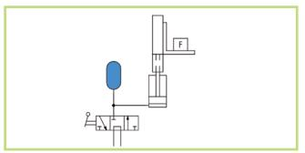
Mechanical shocks occurring for instance when driving on road bumps or obstacles can be absorbed by hydraulic accumulators (e.g. snowploughs). Damping shocks leads to safer manoeuvring and the material is less taken into contribution. Higher vehicle speeds, reducing the risk of accidents, extended equipment service life represent additional advantages.
