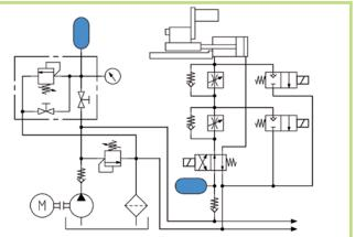
Cutting, advance and retraction speeds, cutting pitch and section of machine-tools with multiple machining units are individually controlled. Therefore, the oil consumption varies significantly. By fitting these machines with an accumulator their irregular oil requirements can be handled guarantying high stating speeds thanks to the low inertia of each oil column compared to those experienced with the complete pumping system.
