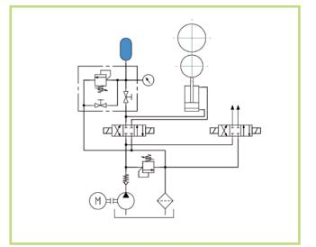
Accumulators can be used to maintain the mechanical pressure applied between two rolls. After having reached the required pressure the pump can be immediately switched to other users, the hydraulic accumulator securing the pressure between the rolls during the entire process.
