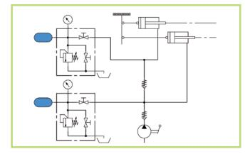
Railway catenaries and suspension cable tensions must be maintained within narrow tolerances. However, the cable length changes as the train passes or depending on the temperature. Accumulators are used for cable length compensation and maintain the cable tension within the prescribed tolerances.
