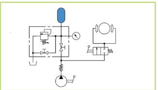
Hydraulic accumulators can for instance be used to control emergency brakes or funicular railway, gondola or bus doors. The accumulators being charged at the station by means of a motorised pump or in emergency case by a hand-pump. The necessary energy is therefor constantly available to carry out an emergency stop.
