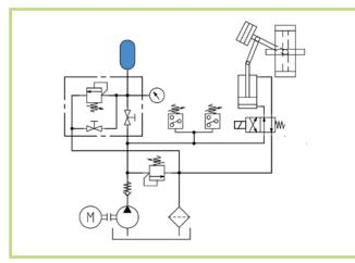
Oil leaks cannot be avoided in hydraulic systems where high pressures have to be maintained for long periods (examples: throttle valves which are maintained open by means of a spring or a counterweight, chucking systems or pressure tests). Oil topping has to be constantly secured.
