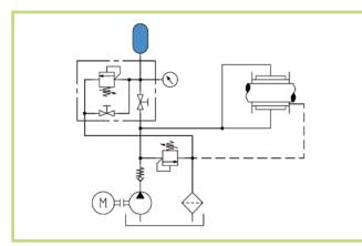
Hydrostatic bearings on machines must be held under pressure. In case of a mains breakdown the pumps stop and the oil pressure falls. OLAER hydraulic accumulators maintain a minimum pressure up to the complete halt of the machine and avoid expensive bearing damages.
