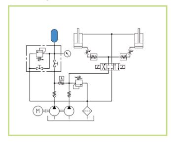
Rational pressing and punching operations are only possible with high-speed empty runs. However, the transformation process must be carried out at low speed and by applying high pressures.
