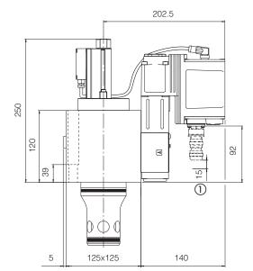
(1) Space to remove the 7 or 12 pin main connector. For main and communication connectors see section 9, 10
