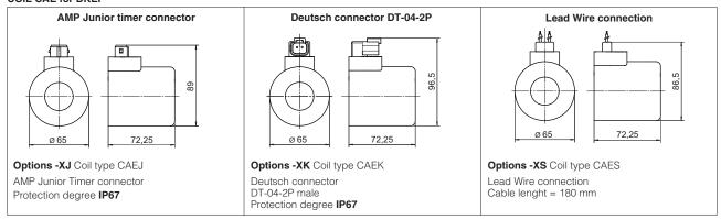
Note: for the electric characteristics refer to standard coils features - see section 6
