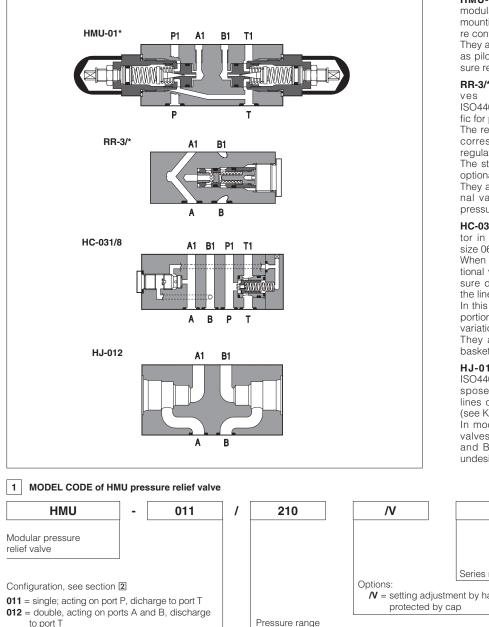
HMU-01 are pressure relief valves in modular execution with ISO4401 size 06 mounting surface, specific for fine pressure control at low flow.
