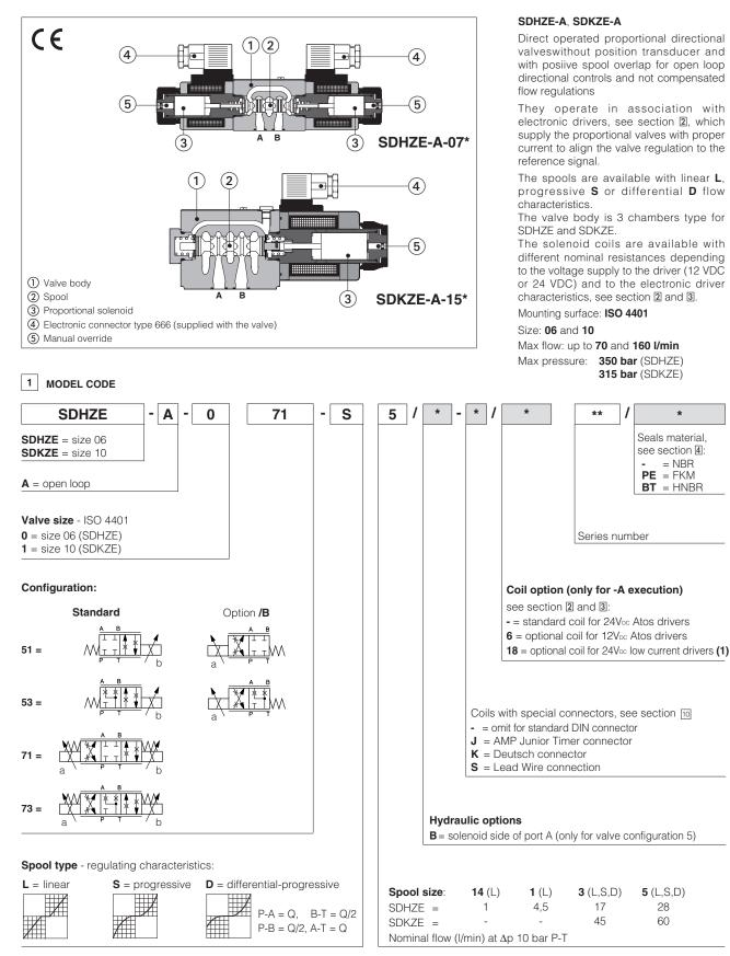
(1) select valve's coil voltage /18 in case of electronic drivers not supply by Atos, with power supply 24Vbc and with max current limited to 1A.
