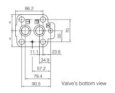
ISO 6264: 2007 Mounting surface: 6264-08-13-1-97 (see table P005) Fastening bolts: 4 socket head screws M16x50 class 12.9 Tightening torque = 300 Nm Seals: 2 OR 4112, 1 OR 109/70 Ports P, T: Ø = 24 mm Port X: Ø = 3,2 mm
