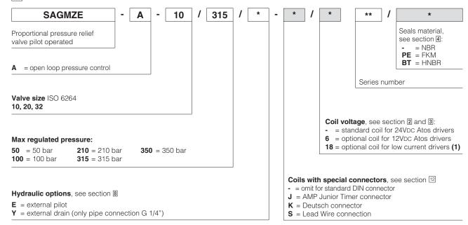
(1) select valve's coil voltage /18 in case of electronic drivers not supplied by Atos, with power supply 24Vpc and with max current limited to 1A.
