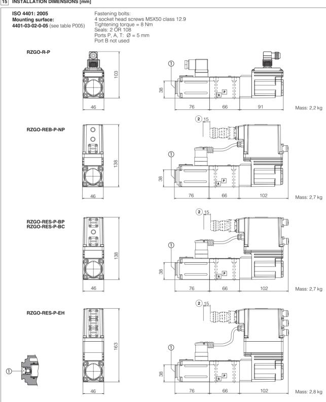
① = Screw for air bleeding: at the first valve commissioning the air eventually trapped inside the solenoid must be bled-off though the screw ①
