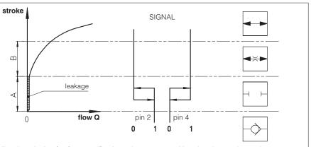
According the criteria of safety specifications, the poppet position signal must change its status inside the overlapping stroke (before the effective valve opening).
