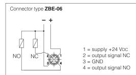
NOTE: the /FV position switch are not provided with a protective earth connection
