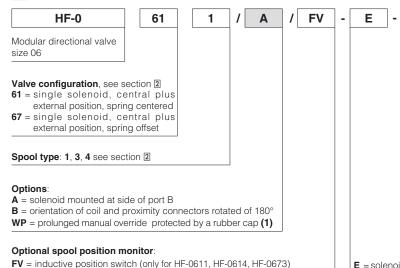
24DC Seals material, see section 4: = NBR PE = FKM Series BT = HNBR (1) number
