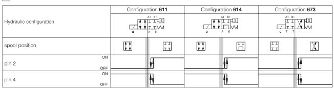
Note: FV position switch can be electrically wired by the customer as NO or NC and then the status of the output signal will be in accordance to the selected configuration
