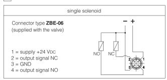
**Note:** the /FV position switch is not provided with a protective earth connection
