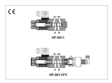
HF are spool type, direct operated solenoid valves in modular execution, normally used for safety functions to shut-off or to by-pass the hydraulic user lines.
