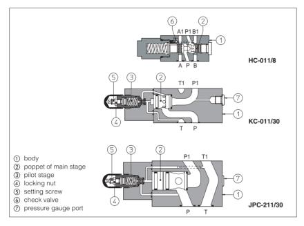
**HC**, **KC** and **JPC** are two way pressure compensators for modular assembling with on/off and proportional directional control valves.
