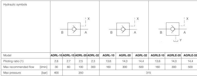
(1) Applying the pilot pressure through the pilot port X, the pilot spool opens the check valve, allowing free flow B→A.
