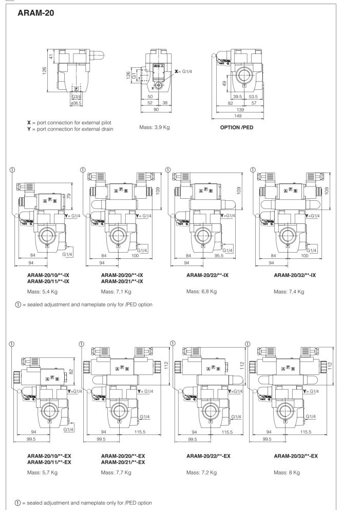
Overall dimensions refer to valves with connectors type 666
