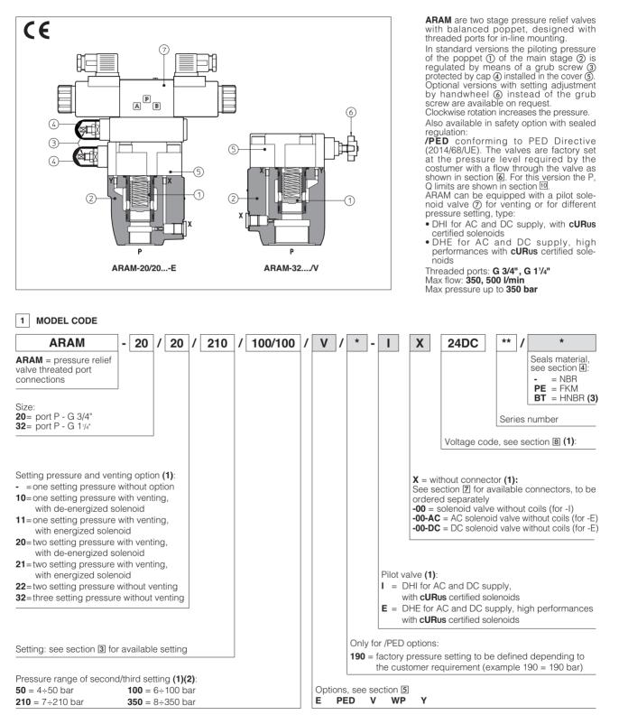
(1) Only for ARAM with solenoid valve for venting and/or for the selection of the setting pressure.
